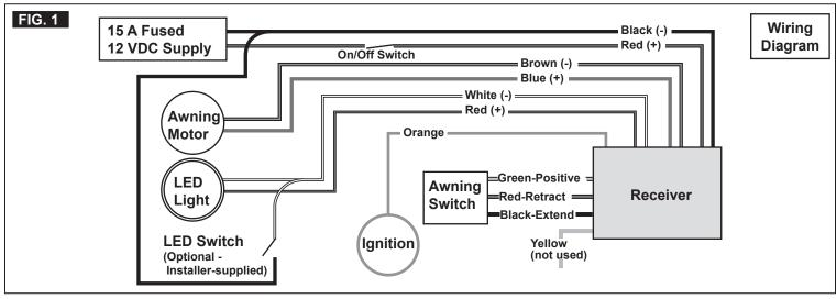
Use the installer-supplied receiver harness connectors, if desired.
